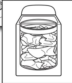
Load garments in loose heaps evenly around the washplate. Do not load garments directly over the center of the washplate; when loaded, the center of the washplate should be visible. Try mixing different sized garments to reduce tangling.
