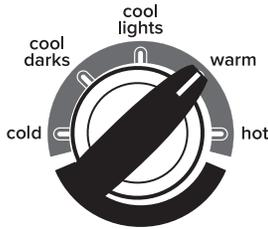
Once you select a cycle, select the desired wash temperature by turning the Wash Temperature knob to the desired setting.
